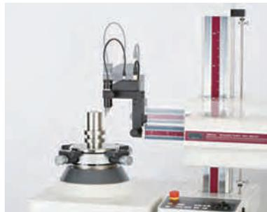
Mesure/analyse spirale (RA-1600)
