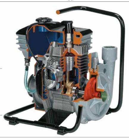
These cutaway models are carefully sectioned for training purposes, professionally painted with different colours to better differentiate the various parts, cross-sections, lubricating circuits, fuel system, cooling system etc. Many parts have been chromium, plated and galvanized for a longer life.
